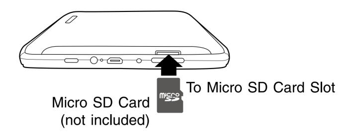
Insert the micro SD card, with contacts facing the screen, into the tablet's Micro SD slot until it clicks.
